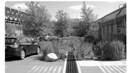
Rain gardens fed by passive rainwater harvesting border the buildings and parking lots of the TAD redevelopment project in Denver, CO. The rain gardens beautify the site, reduce the urban heat island effect, and provide habitat, while reducing runoff to the nearby South Platte River. Photo courtesy of Brook Associates.
