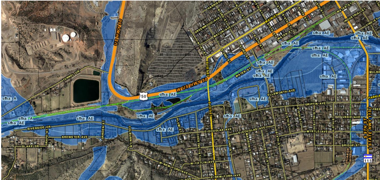
Figure 5: 100 Year flood extent of inundation through Cañon City (Fremont County, 2016)
