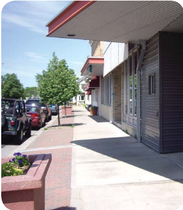
Image illustrating a wider simple amenity zone with special paving to denote the zone. Notice that this and several of the upcoming examples have on-street parking.
