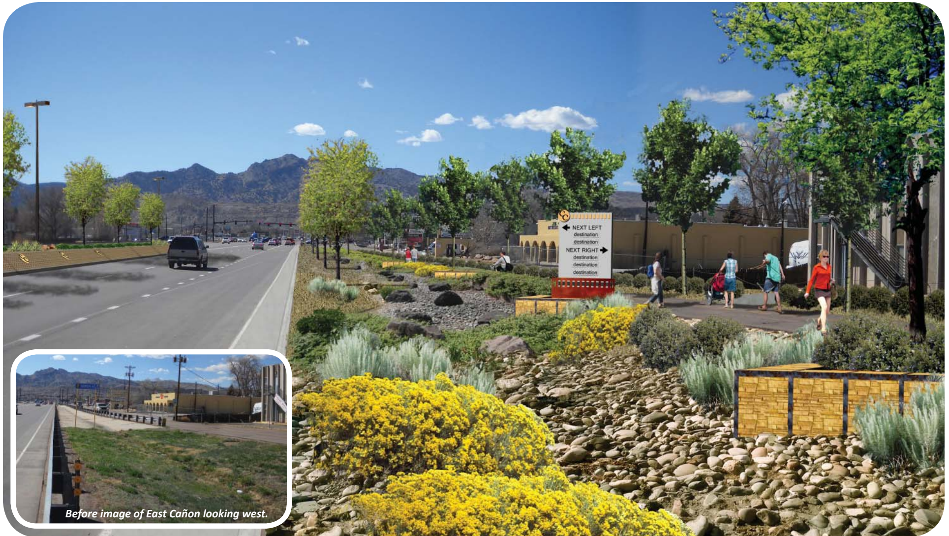
Illustrative rendering showing a proposed East Cañon condition looking west at Cottonwood Avenue: frontage road removed, improved drainage, landscaping, and signage.
