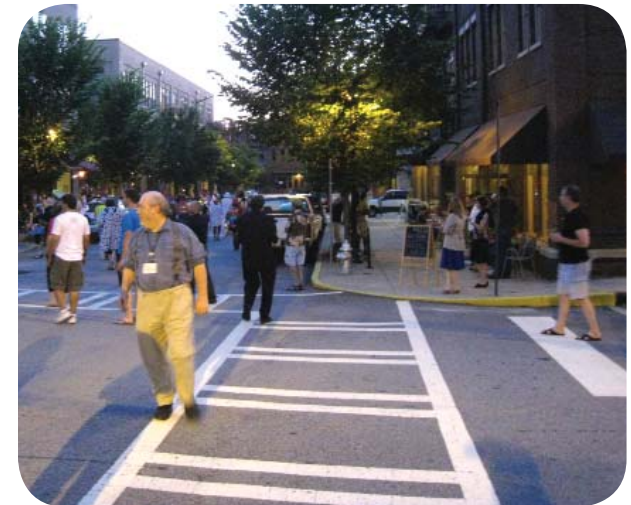
Image of clearly striped pedestrian crossing area and vehicle stop bar. Paint is inexpensive and critical to maintain in crosswalks.
