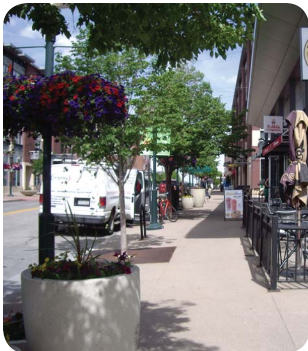
Image illustrating a generous back of curb to building face environment that allows for an amenity zone, clear zone, and cafe zone.
