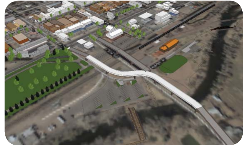
Diagram illustrating in grey the existing alignment of the 4th Street bridge, and in white, a proposed alignment with 3rd Street at RGB, if feasible.
