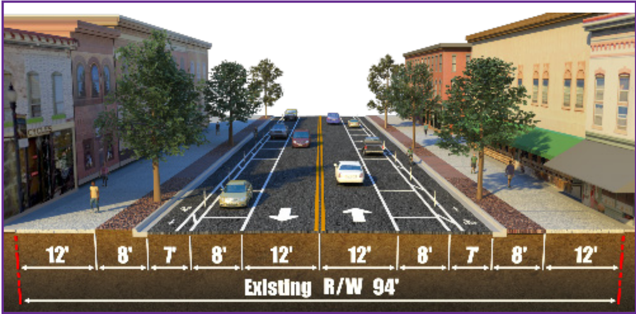
Figure 5.14 Main Street Typical Section 3
